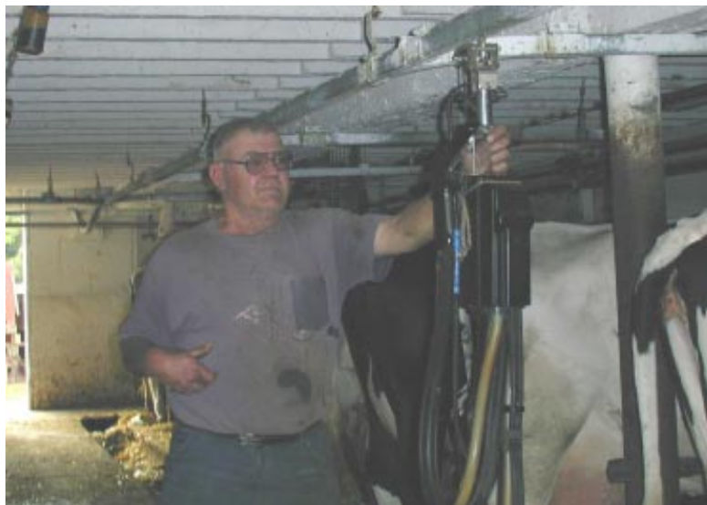
Richard Maurer, Perry County, Pennsylvania uses a new track system in his dairy operation. It makes it easier for him to move the milking unit between cows, and it is equipped with automatic take-off units.
