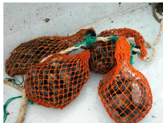
Figure 2. Buoy-line assembly and attached mussel-filled bags
