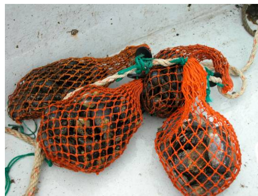
Figure 2. Buoy-line assembly and attached mussel-filled bags
