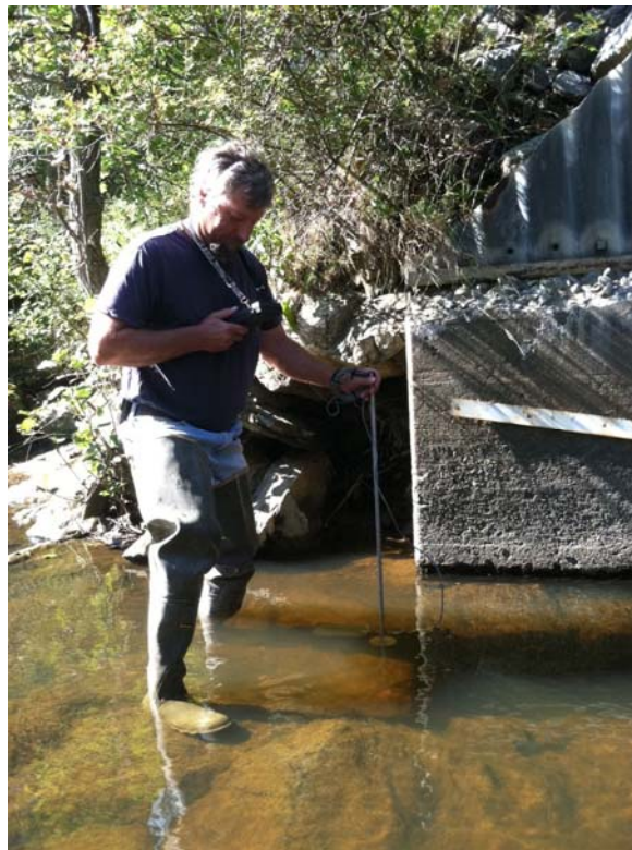
Figure 4. Measuring water level at established staff gauge
