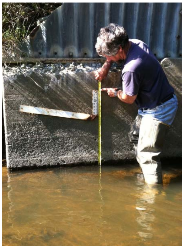
Figure 4. Measuring water level at established staff gauge
