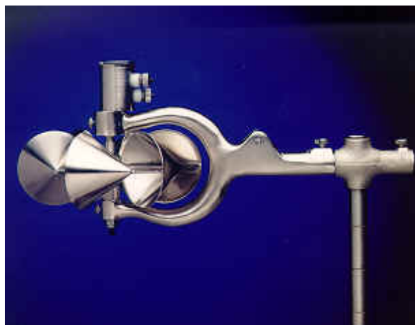
Figure 1. Gurley Price Type AA flow meter (image/specifications table source: Gurley Precision Instruments http://www.gpi-hydro.com/ )
