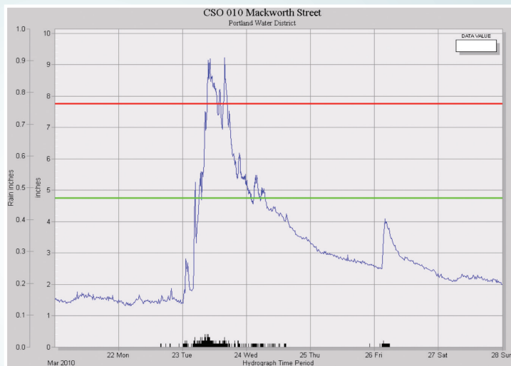
Example monitoring data from the monitored CSO at Mackworth Street. Vertical axis shows inches of water in the pipe, a measure which is directly related to flow. The site alerts PWD staff when the water reaches slightly less than five inches (green line), even though an actual CSO would occur only when the water depth rises to nearly eight inches (red line). (The data are from March 2010.)
