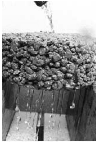
Water flowing through pervious concrete
